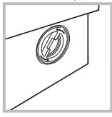
1. unscrew the lid rotating it anti-clockwise (see figure): a little water may trickle out. This is perfectly normal;
